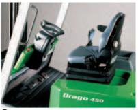
$S_{ ext{pace}}$  for the operator. The cab provides wide space to the driver and a clear view when manoeuvring. The truck may be fitted with pedal direction control to suit all driving styles.
