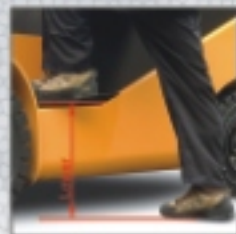
Safe and easy access is assured by a large, non-slip step and grab handle.
