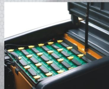
Full accessible 48 volt batteries with 400-600 Ah capacity are controlled by either ZAPI SEM or Danaher AC control systems.
