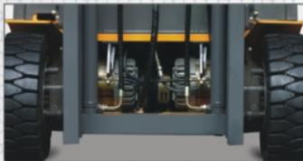
Front-wheel drive through two drive motors incorporated in a compact axle. DC or AC motors are used, depending on truck size and workloads.
