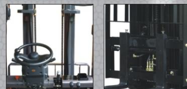
The wide mast, low scuttle and high seating position gives the operator an excellent view of the forks and of the way ahead-reducing load damage and accidents.
