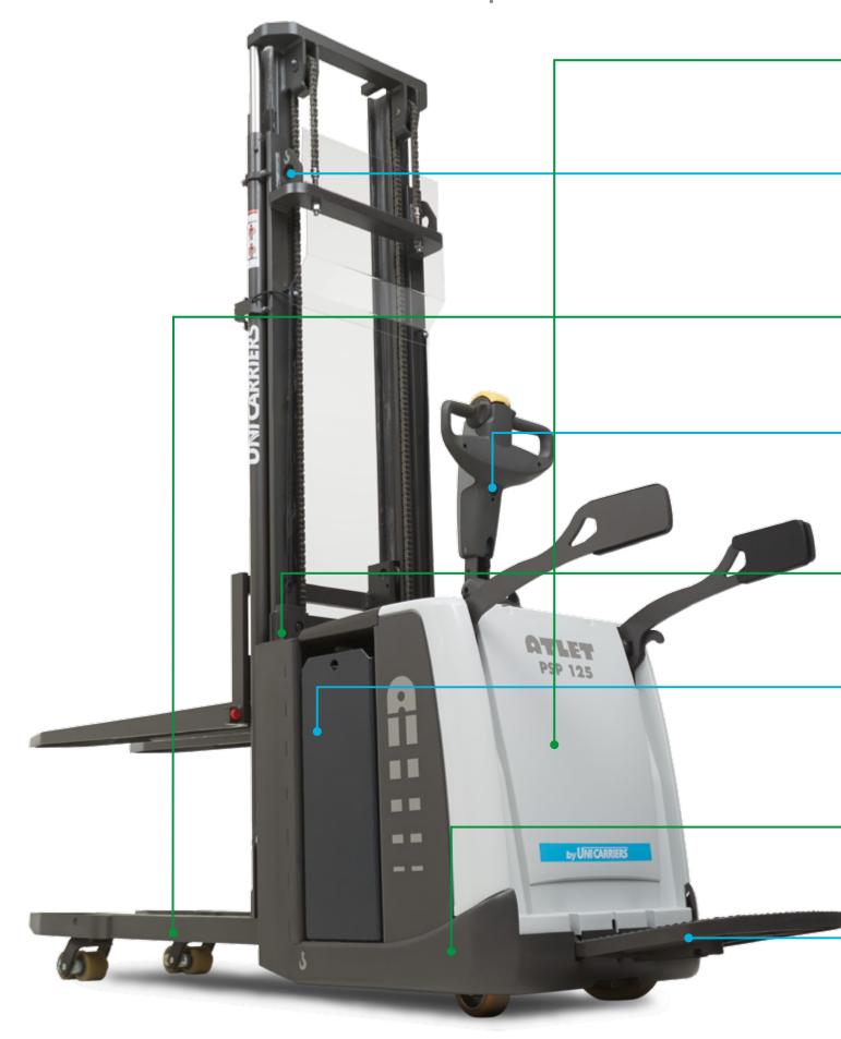
ProVision mast design with off-centre lift cylinder for optimised vision over forks.
