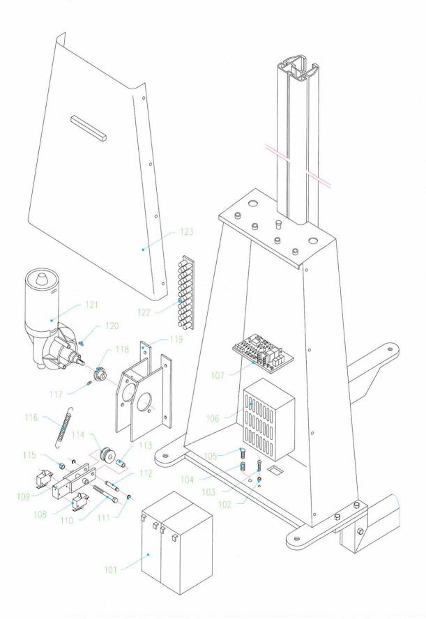
2. E80 Electric Box of Single Pole Elevator Explosive Graphics
