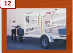
Self driving system in pole. With batteries and charge.
