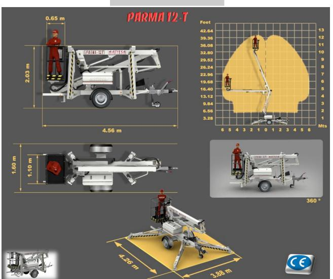
Number of persons - 2 Working height - 12m Maximum outreach - 6,1m Maximum capacity - 200kg Gross weight C.A. - 1.450kg Gross weight C.C. - 1.510kg Rotation - 360° Motor 220V C.A. - 1,8kw
