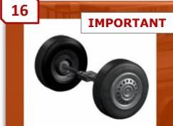
Fixed axle: added when the weight of the selected accessories is exceeded.
