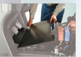
One-Piece, No-Tool Floorboard One touch removal of the diamond tread floorboard gets you right to service operations
