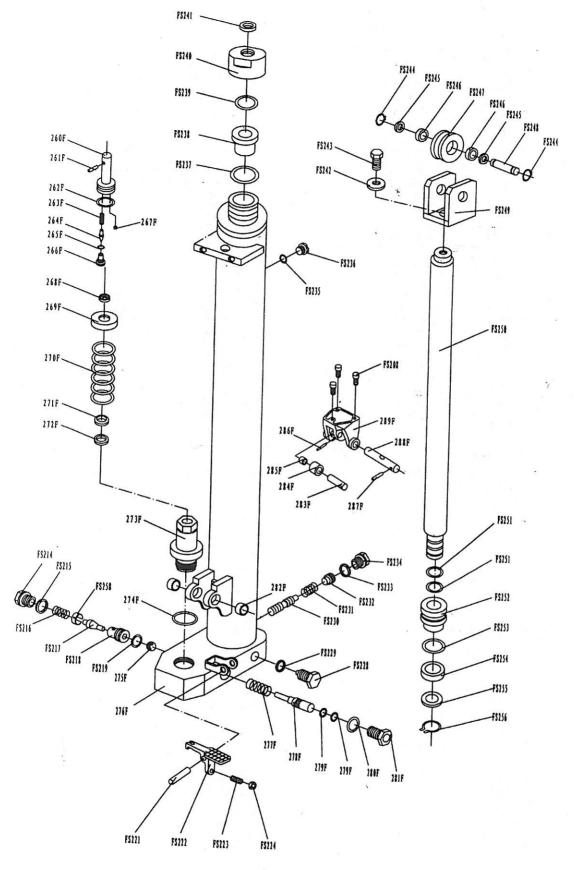
**Pump Part List for Fast Lifting**
