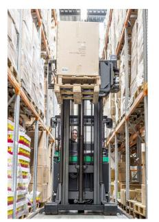
Its market-leading performance with top speeds of up to 14 km/h combined with ergonomic design and comprehensive safety features make for high productivity through incredibly efficient, safe operation. When outside of aisles, VNA trucks can often be less efficient and
