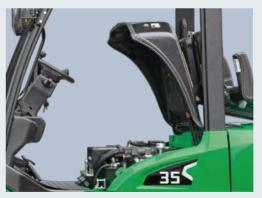
The hood can be opened at a large angle facilitating the maintenance.
