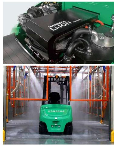
IPX4 water resistance rating, suitable for outdoor operation
