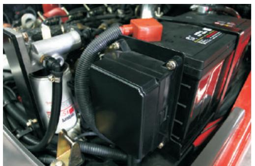
CUMMINS engine use the special air filter, it can reduce air intake resistance dramatically, equipped with pressure alarm to master the maintaining time.
