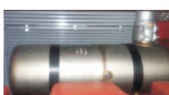
The exhaust treatment DOC ensure the exhaust satisfy with Europe 3B and USA T4F , it also with good noise reduction , maintenance is minimal.
