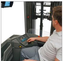
Equally capable of handling long loads and standard pallets, the RBM20-25N3 Series offers lift heights up to 9.7 metres. As it's four-way and can carry long loads sideways, aisles can be kept to a minimum, allowing you to maximise storage space.
