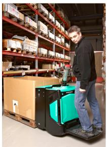
PREMiA Es models have an exceptionally short chassis for working in very narrow aisles, allowing maximum storage density. It's marketleading lift height and linked castor wheels ensure stability when operating on ramps, loading docks and uneven surfaces.
